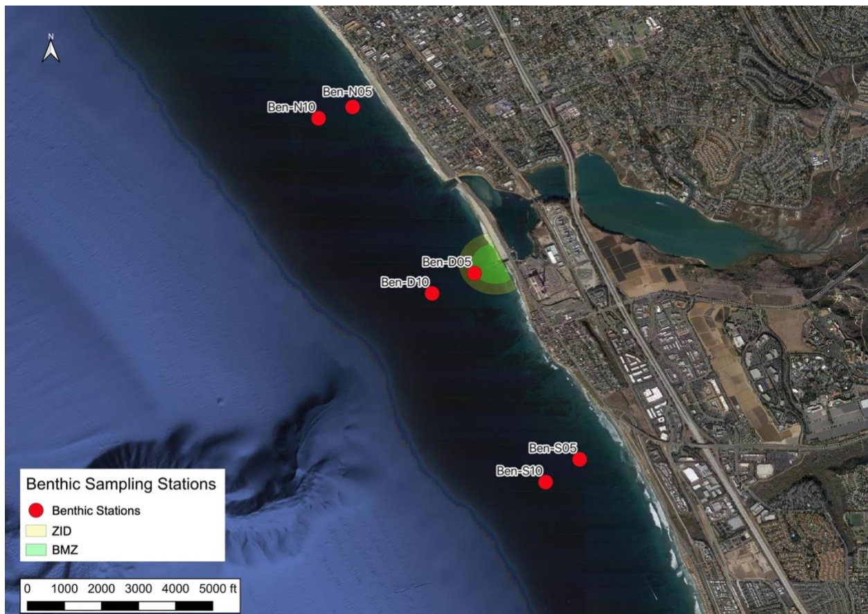
Figure 4. Carlsbad Desalination Plant benthic sampling stations in relation to the discharge channel, brine mixing zone (BMZ), and zone of initial dilution (ZID).
