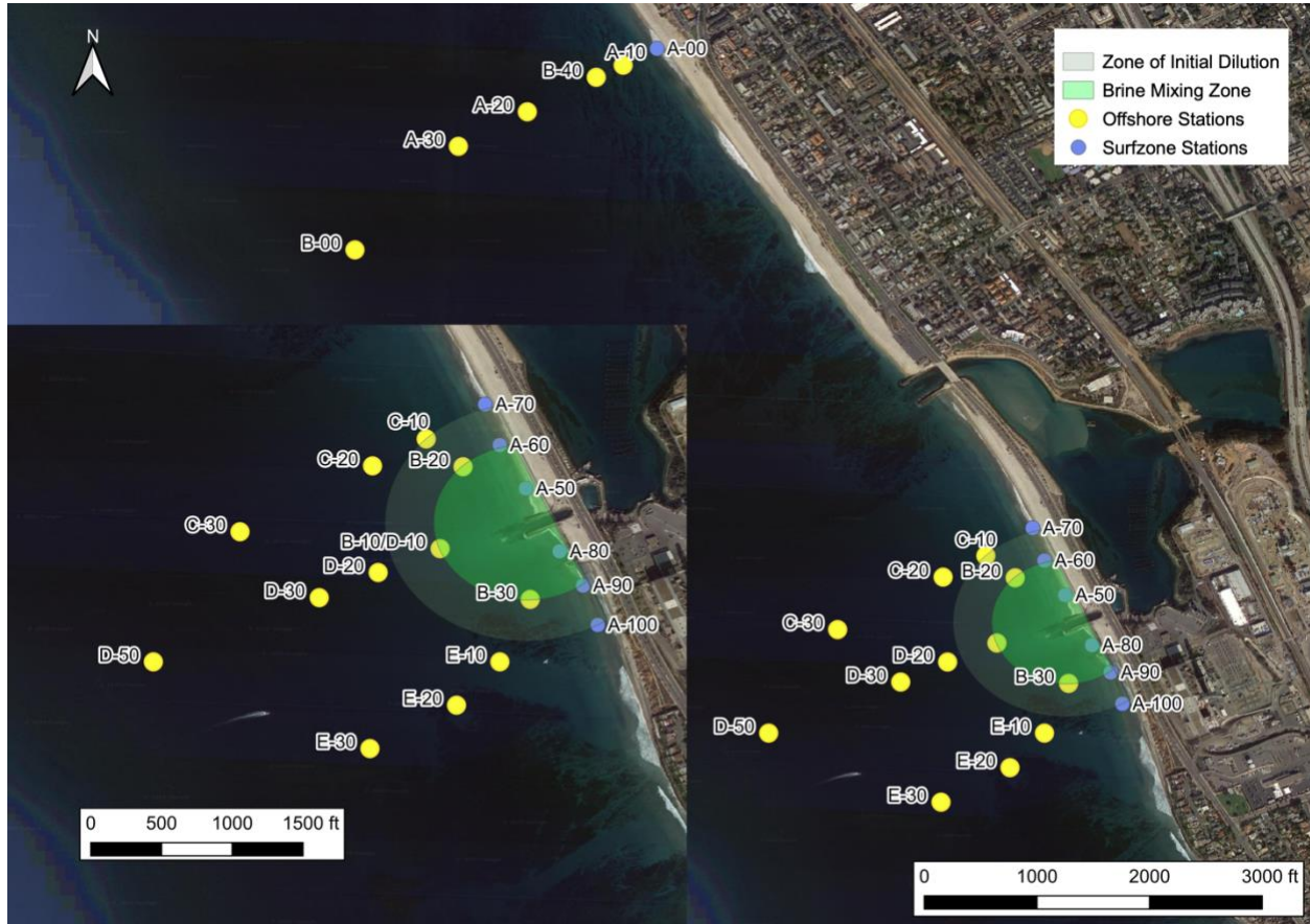
Figure 2. Water quality stations monitored in compliance with Order No. R9-2019-0003 for receiving water quality. The Brine Mixing Zone and Zone of Initial Dilution are both depicted.
