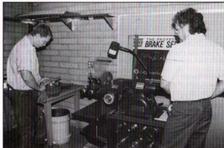
Equipment Mechanics Rick Burke and Mike Staley machine surface brake drums and rotors on a newly acquired brake lathe.
