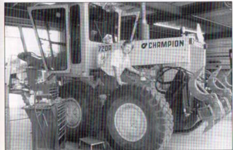
Equipment Mechanic Mike Staley performs a major service on Authority motor grader.
