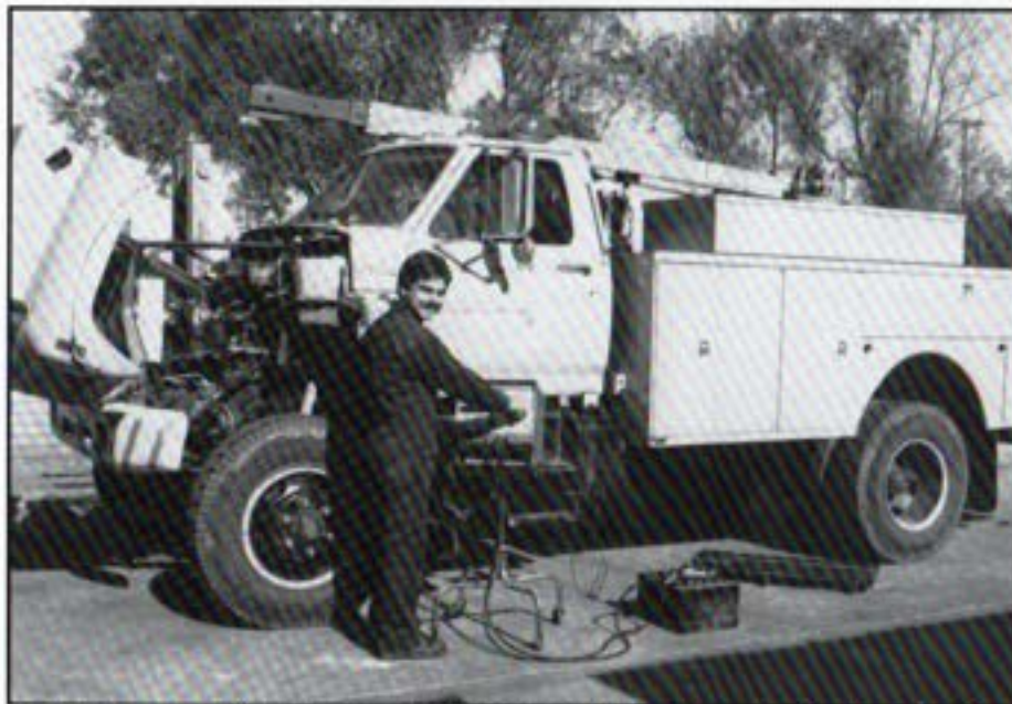
Al Garza, an equipment shop mechanic, troubleshoots an electrical problem in this valve service truck.
