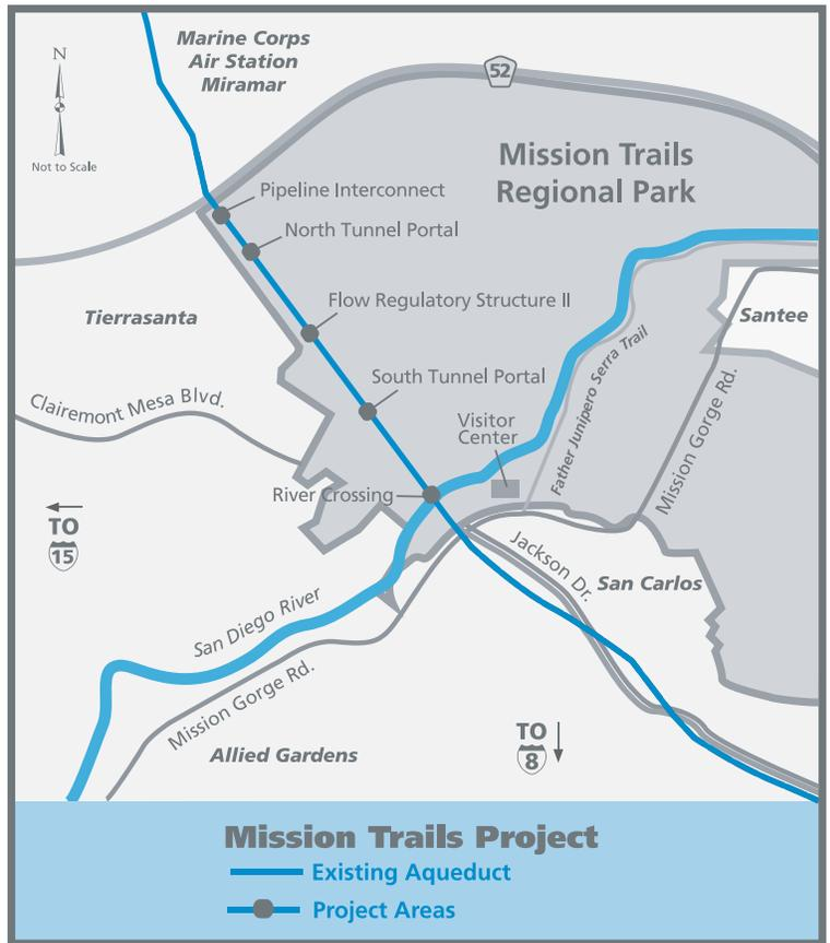
in the same area of the park in the mid-1990s. The new underground tank will contain up to 12 million gallons of water. An access building will be constructed above ground for maintenance and operation purposes. Flow regulatory structure construction is anticipated to begin in mid-2011 and last approximately two years.
