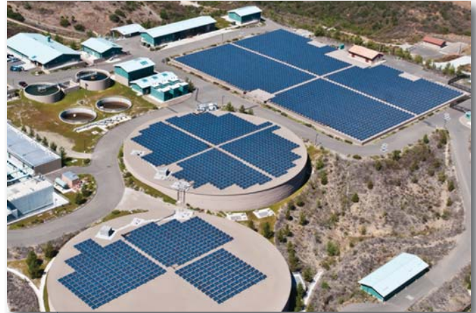
Photo courtesy of Borrego Solar Systems, Inc. Solar panels at Twin Oaks Valley Water Treatment Plant.
