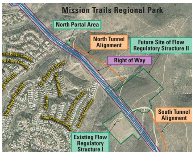
Mission Trails Project tunnel alignment.
