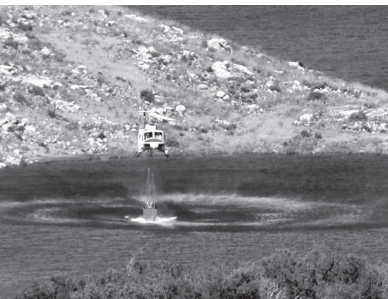
Helicopter bucket scoops reservoir water to extinguish flames.
